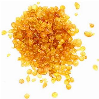
Bone glue, made of animal bones, as the name suggests, was in general use among cabinetmakers for centuries. Bone was ground into powder, dissolved in water, evaporated and dried into a hard jelly. Bone glue is completely safe and environmentally benign.
